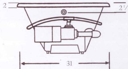
ELECTRICAL REQUIREMENTS: 115V, 20 AMP, GFCI Protected Circuit.
