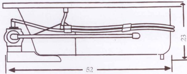
PUMP MOTOR: Standard 1/4 HP, Single Phase, 115V, 60HZ, 3425 RPM, Pre-installed (factory)
