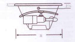
PUMP MOTOR: Standard  $1^{1/4}$  HP, SIngle Phase, 115V, 60HZ, 3425 RPM, Pre-installed (factory)
