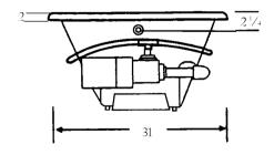
PUMP MOTOR: Standard 1.74 HP, Single Phase, H5V, 60HZ, 3425 RPM, Pre-installed (factory)
