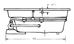
PUMP MOTOR: Standard 1  $^{1/4}$  HP, SIngle Phase, 115V, 60HZ, 3425 RPM, Pre-installed (factory)
