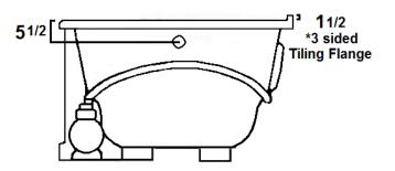
Standard (S) Pump Location and Alternate (A-1 & A-2) Pump locations. \* Pump location if Heater ordered.
