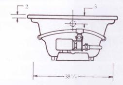
PUMP MOTOR: Standard  $1\,{}^{1}\!/_{\!\!4}$  HP, SIngle Phase, 115V, 60HZ, 3425 RPM, Pre-installed (factory)
