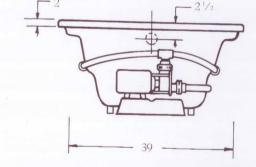
PUMP MOTOR: Standard  $1^{1/4}$  HP, SIngle Phase, 115V, 60HZ, 3425 RPM, Pre-installed (factory)
