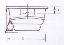
PUMP MOTOR: Standard 1<sup>1</sup>/<sub>4</sub> HP, SIngle Phase, 115V, 60HZ, 3425 RPM, Pre-installed (factory)
