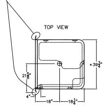
ROUGH IN DIMENSIONS FOR UNITS WITHOUT SEAT FEATURED: 38 1/4" x 37 1/4" x 82 7/8" ROUGH IN DIMENSIONS FOR UNITS FEATURING A MOLDED SEAT: 38" x 37 1/4" x 82 7/8" ROUGH IN DIMENSIONS FOR UNITS FEATURING A FOLD UP SEAT: 39 3/4" x 37 1/4" x 82 7/8" \* NOTE: THIS DIMENSION IS NOT TO SCALE. THIS DIMENSION INCLUDES NUTS/BOLTS, WOOD AND HARDWARE REQUIRED FOR ASSEMBLY. OFFSET THE 39 3/4", 1/2" TOWARDS THE FOLD UP SEAT SIDE TO ALLOW FOR THE BOARD.
