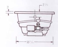
PUMP MOTOR: Standard 11/4 HP, SIngle Phase, 115V, 60HZ, 3425 RPM, Pre-installed (factory)
